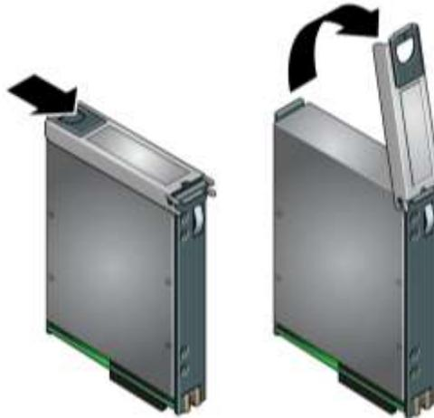
4. Hold the disk drive by the plastic carrier and position the disk drive so that the latch is toward the rear of the array (where the power supplies and control modules are). Start to insert the drive (1).
