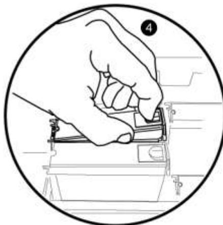
8. Holding the latch open, lower the lever until the drive is fully seated and flush with the other drives (5). Keep holding the latch open.
