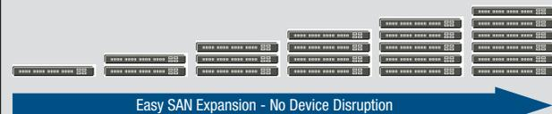
*Need more server or storage ports? Simply add another switch to the stack – no need to move existing cables or to disrupt devices. It's like having the performance and hands-off convenience of an expensive chassis switch, without the cost overhead of a chassis!*
