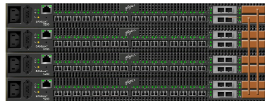
Four switches for 64 ports
